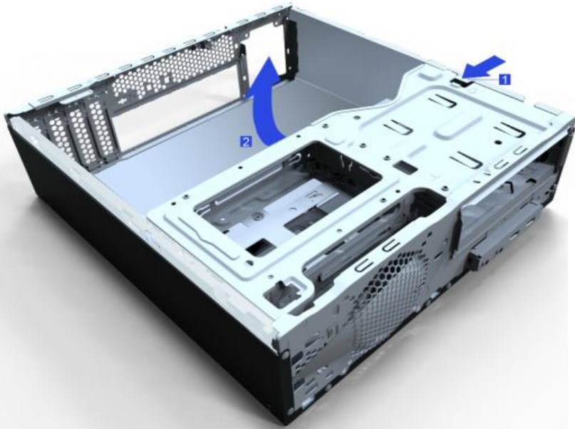
Pivoting the drive bay assembly upward
